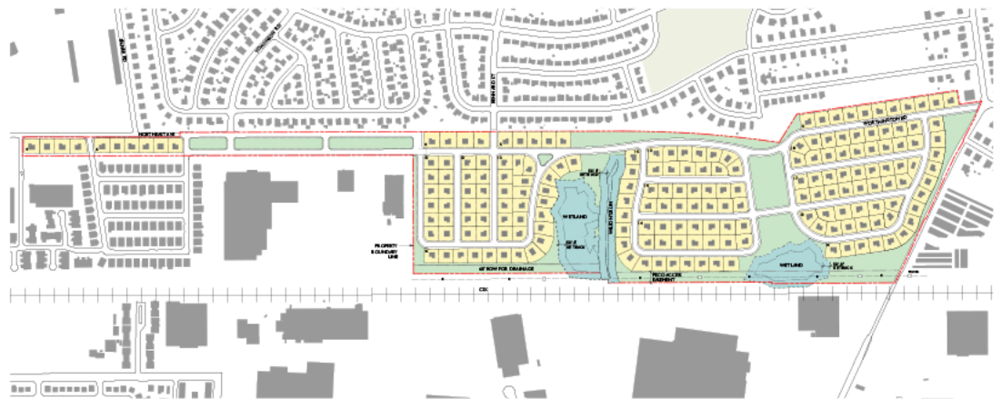
The master plan creates three residential hubs organized off a central boulevard and separated by open space and wetlands.
